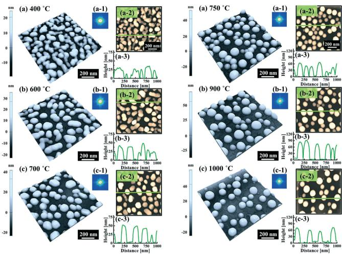
Fig. 5 Evolution of Au nanostructures by the variation of annealing temperatures between 400 and 700 °C on 4H-SiC (0001). Each sample is fabricated with a fixed deposition amount of 8 nm and an annealing duration of 450 s. (a)–(c) AFM side-views of  $1 \times 1 \mu m^2$ . (a-1)–(c-1) 2D FFT power spectra. (a-2)–(c-2) AFM top-views of 1  $\times$  1  $\mu$ m<sup>2</sup>. (a-3)–(c-3) Cross-sectional line profiles.
