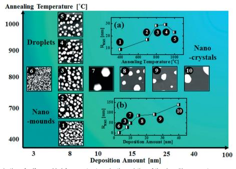
Fig. 8 Map of the fabrication of self-assembled Au nanostructures by the variation of the deposition amount *versus* annealing temperature. (a)  $R_{\text{RMS}}$  of the samples synthesized with 8 nm Au deposition at various annealing temperatures. (b)  $R_{\text{RMS}}$  of the samples with various deposition amounts annealed at 800 °C for 450 s. Insets:  $1 \times 1 \, \mu\text{m}^2$  for 1–7 and  $3 \times 3 \, \mu\text{m}^2$  for 8–10.
