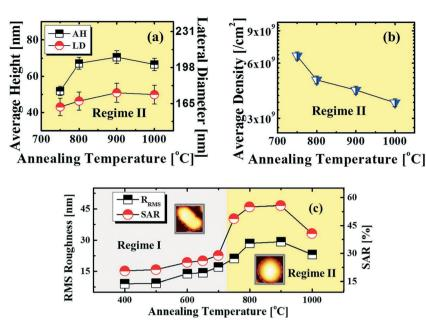
Fig. 7 (a)–(b) Plots of the AH, LD and AD with error bars of  $\pm 5\%$ . (c) Plot of  $R_{\rm RMS}$  and the surface area ratio (SAR). The SAR is  $(\beta - \alpha)/\beta \times 100$  (%), with a surface area ( $\alpha$ ) of  $x \times y$  and a geometric area ( $\beta$ ) of  $x \times y \times z$ . Insets: two AFM top-views in (c) are 150  $\times$  150 nm<sup>2</sup>.
