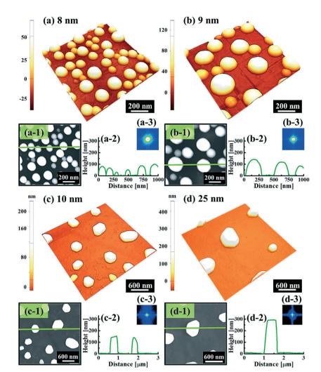
Fig. 2 Shape transition of the self-assembled Au nanoparticles on 4H-SiC (0001) by the variation of deposition amounts between 8 and 25 nm under identical growth conditions (800 °C, 450 s). AFM side-views of (a)–(b)  $1 \times 1 \mu m^2$  and (c)–(d)  $3 \times 3 \mu m^2$ . AFM top-views of (a-1)–(b-1)  $1 \times 1 \mu m^2$ and (c-1)-(d-1)  $3 \times 3 \mu m^2$ . (a-2)-(d-2) Cross-sectional line profiles acquired from the green lines drawn in (a-1)-(d-1). (a-3)-(b-3) 2D FFT power spectra
