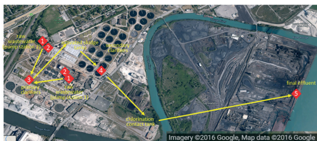
Fig. 1 Aerial view of Detroit WWTP with five sampling locations for the liquid stream: 1) raw wastewater (Jefferson and Oakwood Interceptors via Pump Station 1 and North Interceptor East Arm via Pump Station 2), 2) preliminary effluent, 3) primary effluent, 4) secondary effluent, and 5) final effluent.
