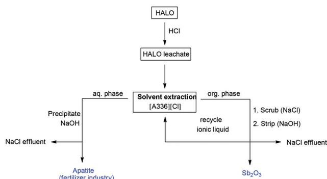
**Fig. 9** Schematic overview of the proposed recycling process. After full dissolution in diluted HCl, the antimony is selective extracted from the leachate using the ionic liquid Aliquat® 336 and pure Sb<sub>2</sub>O<sub>3</sub> is obtained after scrubbing and stripping. The remaining elements in the leachate are then precipitated as an apatite which can serve as feedstock in the fertilizer industry. The only waste of this process is an aqueous NaCl effluent which can be discarded in the sea.
