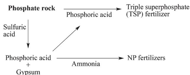
**Fig. 1** Main industrial production routes for phosphate fertilizers.
