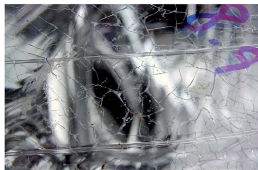
Fig. 4 Liquid medium effect on the headlight lens. 22
