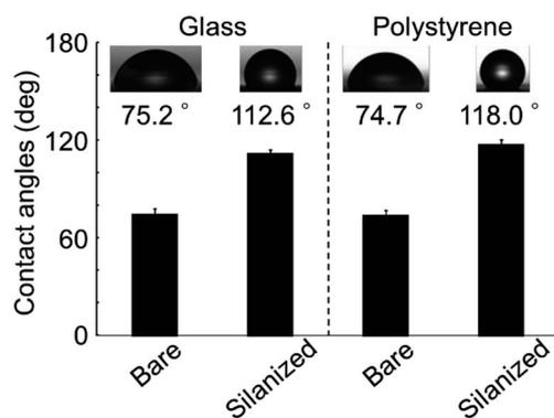
Fig. 4 The contact angles on the bare or silanized cell culture surfaces of both glass and polystyrene. The photographs in the graph show droplets of deionized water on the surfaces. The data bars and error bars indicate the mean values and standard deviations, respectively ( $n = 5$ ).
