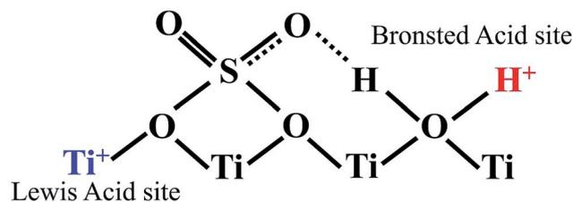
Fig. 7 Illustrative structure indicates the presence of both Bronsted and Lewis acid sites on the surface of TiO<sub>2</sub>–SO<sub>4</sub>.
