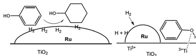
Fig. 3 Illustration of large Ru particles on a TiO<sub>2</sub> support interacting with the aromatic ring and facilitating hydrogenation (left), while small Ru particles create a bifunctional catalyst with the phenyl ring and promote hydrodeoxygenation (right) (adapted from ref. 49).
