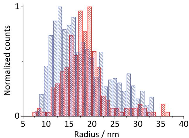
Fig. 4 Histogram of particle radius determined from spikes obtained during chronoamperometry at  $-0.4$  V vs. Ag/AgCl and corrected for the diffusion coefficient (blue, dense mesh) and from TEM (red, medium mesh). The mean value of  $15.2 \pm 1.8$  nm is determined from a log-normal distribution curve of radius resulting from the particle impact.
