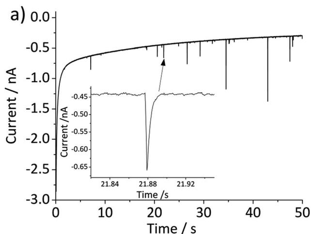
Fig. 3 Characteristic chronoamperogram recorded at a gold micro-electrode in deoxygenated 20 mM KCl with pre-dispersed hematite nanoparticles at pH 2.1 and at an applied potential of  $-0.4$  V vs. Ag/AgCl. The inset provides an enlarged view of the current–time profiles illustrating the faradaic reduction of nanoparticles upon collision with the working electrode as spikes.
