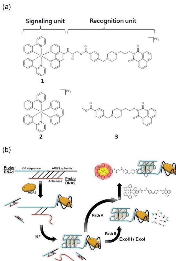
Fig. 1 (a) Chemical structure of Ir(III) complexes **1** and **2** and the G-quadruplex loop binder **3**. (b) Schematic diagram illustrating the AGR2 sensing platform utilizing the DNA binder linked Ir(III) complex **1**.
