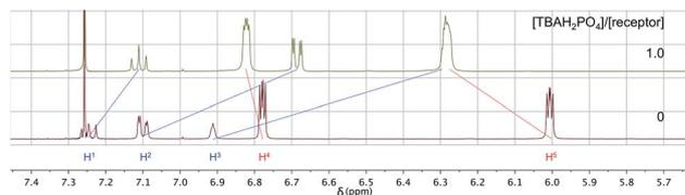
Fig. 6 Partial  $^1\text{H}$  NMR spectra of receptor **4b** before (bottom) and after (top) addition of one molar equivalent of  $\text{TBAH}_2\text{PO}_4$  in  $\text{CDCl}_3$ . Dashed lines show the changes in the chemical shifts of selected proton signals ascribable to receptor **4b**.
