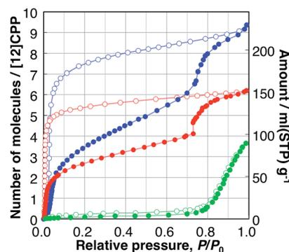
Fig. 2 Adsorption (filled circles), and desorption (open circles) isotherms of H<sub>2</sub>O (green), MeOH (blue), and EtOH (red) on [12]CPP measured at 298 K.
