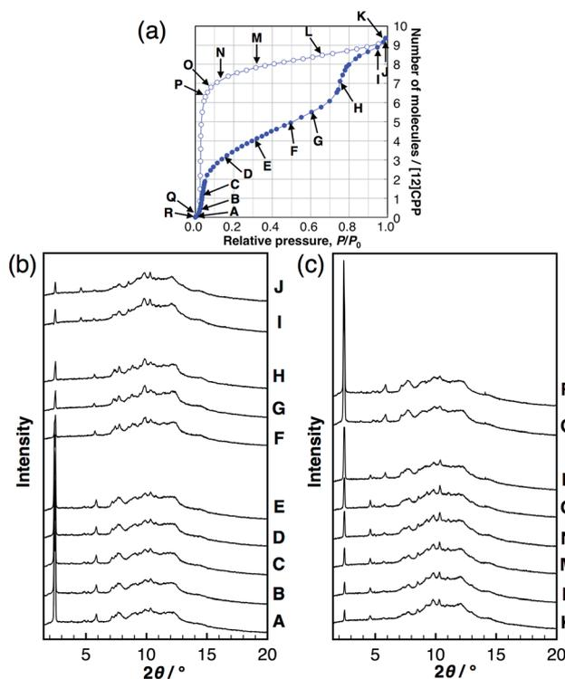
Fig. 3 (a) Adsorption/desorption isotherm of MeOH on [12]CPP at 298 K. Synchrotron powder XRD patterns during (b) adsorption and (c) desorption at the vapor pressures indicated in the isotherm ( $\lambda = 0.79836 \text{ \AA}$ ).
