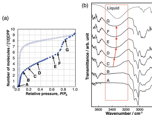
Fig. 5 (a) Adsorption/desorption isotherm of MeOH on [12]CPP at 303 K. (b) IR spectra during the adsorption process at the vapor pressures that are indicated in the isotherm.
