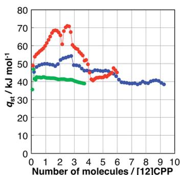
Fig. 4 Isosteric heat of adsorption ( $q_{st}$ ) versus the adsorption amount of H<sub>2</sub>O (green), MeOH (blue), and EtOH (red).
