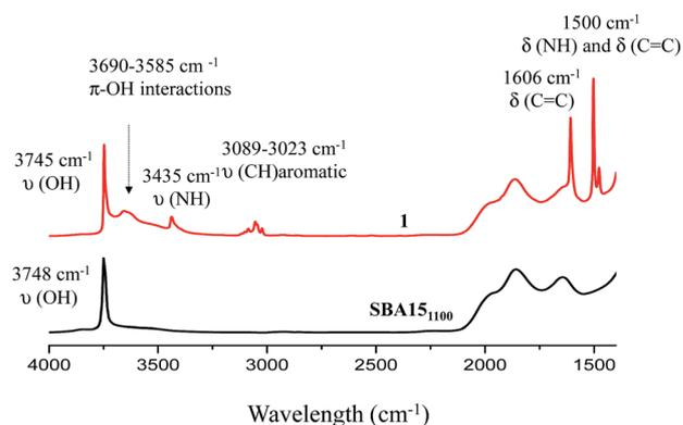
Fig. 1 FT-IR spectra of SBA15<sub>1100</sub> (black) and **1** (red).
