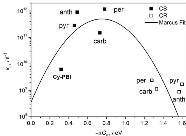
Fig. 5 Plot of electron transfer rate constants in the PBI cyclophane and the corresponding host–guest complexes vs. the thermodynamic driving force ( $-\Delta G_{ET}$ ) for charge separation (solid squares) and charge recombination (open squares); the line represents the fit according to eqn (3) with  $\lambda = 0.75$  eV and  $V = 15$  cm<sup>-1</sup>.
