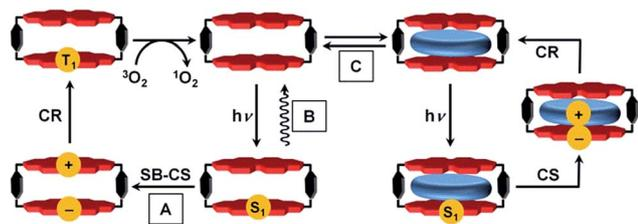
Fig. 1 Schematic of the different excited state photophysics upon excitation; (A) symmetry-breaking charge separation and recombination to the PBI triplet within the PBI cyclophane **Cy-PBI**, in  $\text{CH}_2\text{Cl}_2$  that can be used for singlet oxygen generation; (B) emission in toluene; (C) encapsulation of aromatic guests and photo-driven charge separation between guest and **Cy-PBI** and charge recombination to the ground state.
