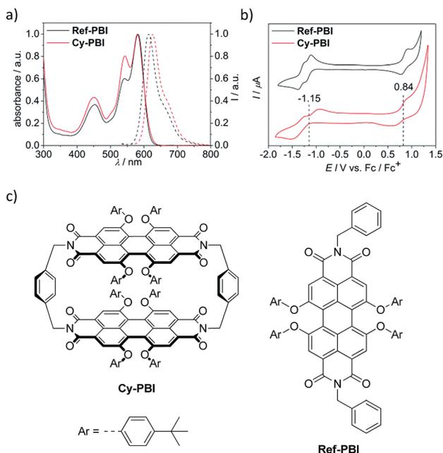
Fig. 2 Normalized UV-vis absorption (solid line) and fluorescence (dashed line) spectra (a) of **Cy-PBI** and **Ref-PBI** ( $\text{CH}_2\text{Cl}_2$ , RT,  $c = 5 \times 10^{-5}$  M); cyclic voltammograms (b) in  $\text{CH}_2\text{Cl}_2$  (reference electrode: Ag/AgCl, working and auxiliary electrode: Pt; 0.1 M TBAHFP,  $\text{Fc}^+/\text{Fc}$ , RT,  $c \sim 2 \times 10^{-4}$  M) and chemical structures (c) of **Cy-PBI** and **Ref-PBI**.
