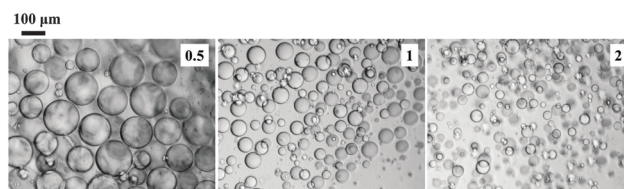
Fig. 9 (upper) Photographs of glass vials containing 50 cS PDMS-in-(a) sunflower oil, (b) olive oil or (c) rapeseed oil emulsions (1 : 1) 1 month after preparation stabilised by different concentrations (given, wt%) of 75% SiOH fluorinated fumed silica particles. (lower) Corresponding optical micrographs of the emulsions in (a) at selected particle concentrations (given, wt%).
