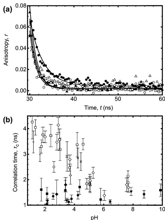
**Fig. 2** (a) Impulse reconvolution fits to the anisotropy function for the same samples (and legend) as shown in Fig. 1a. As in Fig. 1a, the large molar mass sample ( $M_n = 63.2$  kDa) showed pH responsive behaviour, with a longer correlation time at pH 3 than the other three samples. The solid lines are fits to the data. (b) Complete correlation time data as a function of pH. The symbols are the same as those in the legend in Fig. 1b.
