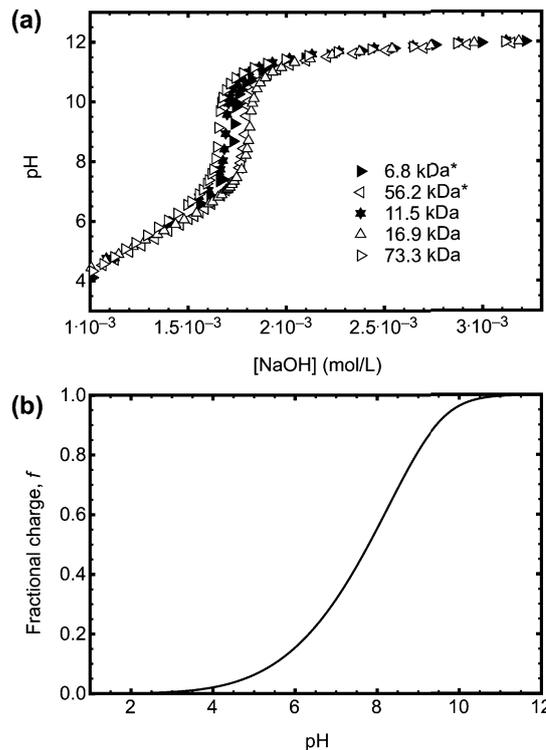
Fig. 4 (a) Potentiometric titration data for a series of PAA samples (initially dissolved in water at a concentration of  $1 \text{ mg ml}^{-1}$ ) with and without (\*) ACE label. The data shown here are for PAA synthesized using CTA **1** (6.8, 11.5, and 56.2 kDa), **2** (73.3 kDa), and **3** (16.9 kDa). The labelled polymers used different RAFT CTAs. (b) Fractional charge calculated from eqn (6).
