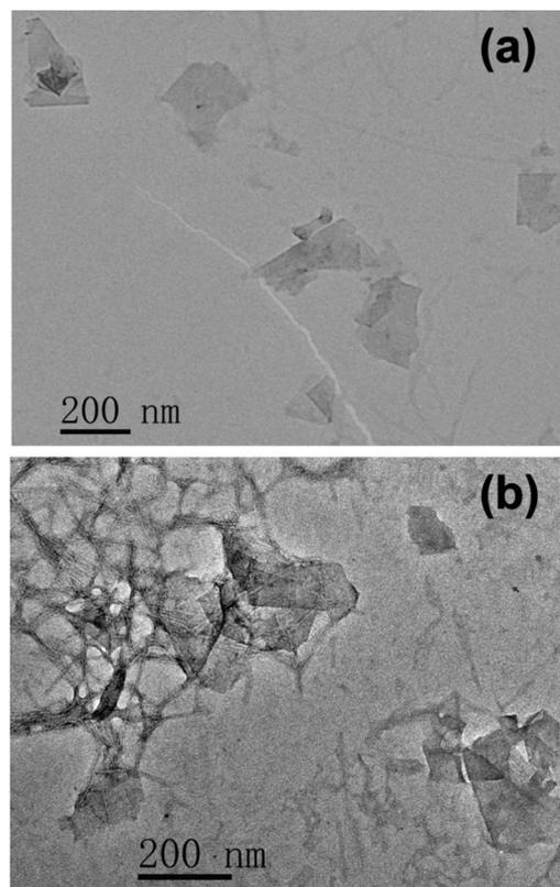
Fig. 5 TEM images of (a) the unstained and (b) the negatively stained samples showing the suspended flake species in the  $I_3C-Cl_3$ -treated graphene dispersion after centrifugation at 5000 rpm for 10 min.
