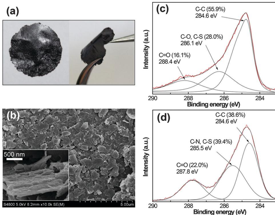
Fig. 8 (a) The photographs and (b) the SEM images (inset, a magnified image) of the graphene/ $I_3C-Cl_3$  composite film prepared by simple filtration of a dispersion through a nylon filter membrane of  $0.22\ \mu\text{m}$  pore size. Note that the dispersion was obtained by centrifugation at 5000 rpm for 10 min. XPS profiles ( $C_{1s}$  spectra) of (c) the graphene/ $I_3C-Cl_3$  composite and (d) the  $I_3C-Cl_3$  powder.
