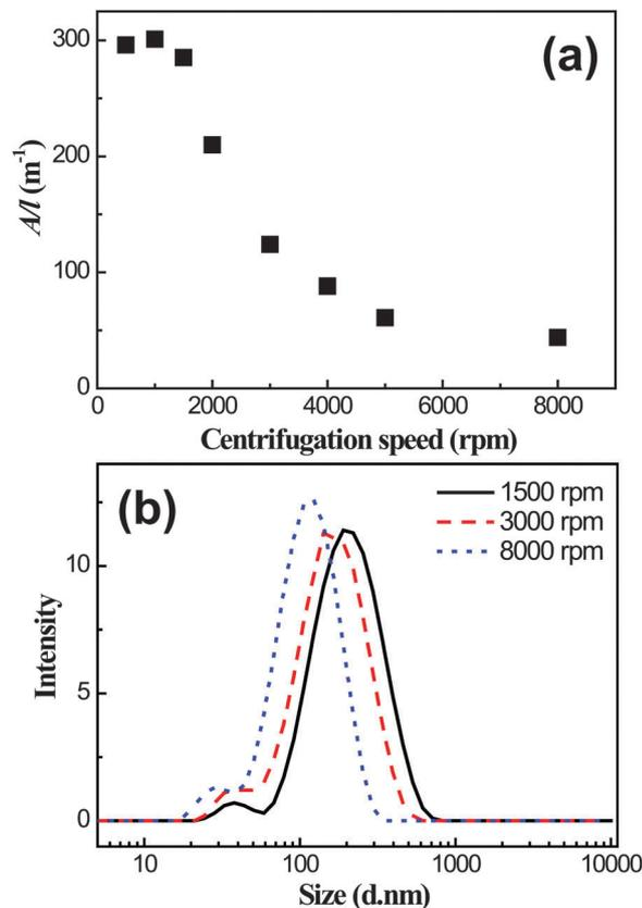
Fig. 4 (a) The  $A/l$  values at 660 nm for the  $I_3C-Cl_3$ -treated graphene dispersions after centrifugation at different speeds for 90 min. (b) Size distributions of the dispersed graphene flakes in solutions centrifuged at different speeds as measured by DLS.
