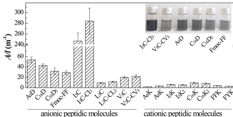
Fig. 2 The  $A/l$  values of the peptide-treated graphene dispersions that were obtained through centrifugation at 5000 rpm for 10 min after sonication in peptide solutions. The inset shows the photographs of several typical dispersions with relatively high exfoliation efficiency.
