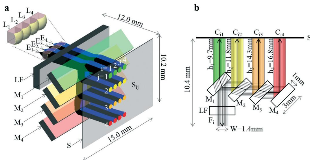
**Fig. 2** Design of the developed ultra-small system with a size of  $15.0 \times 10.2 \times 12.0$  mm. (a) Perspective view overlaying ray-trace simulation fluxes of rays emitted from  $E_i$  (black lines are rays from  $E_1$  and  $E_3$ , and blue lines are rays from  $E_2$  and  $E_4$ ); LF: long-pass filter;  $S_{ij}$ : image of  $C_{ij}$ . (b) Cross-sectional view overlaying complete parallel light fluxes;  $h_j$ : sensor distances for color number  $j$ ;  $W$ : aperture of the system.
