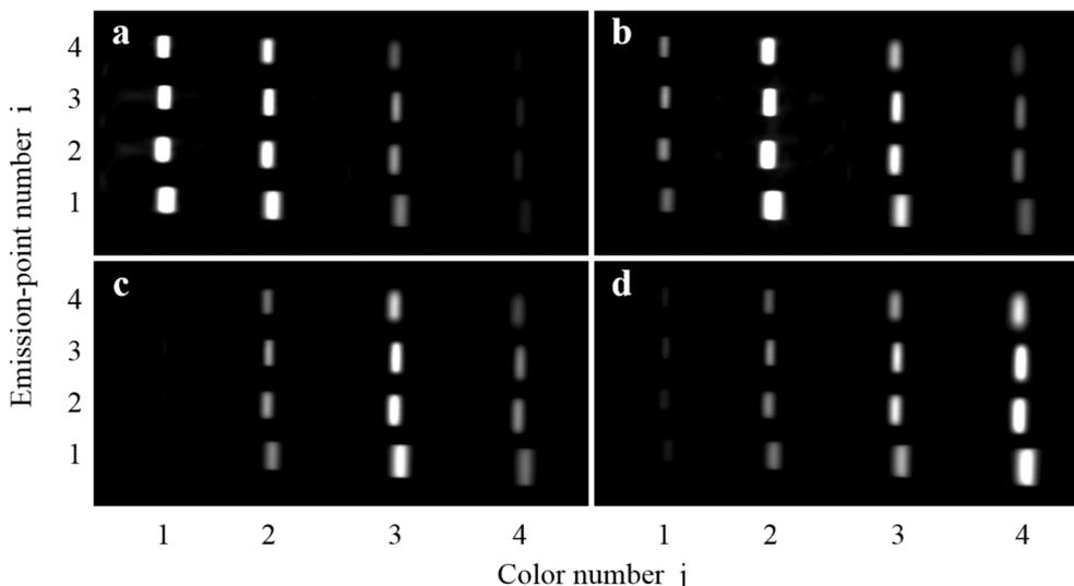
**Fig. 6** CMOS images obtained by the developed ultra-small optical system for 8 M urea solutions containing (a) 100 nM dR110, (b) 100 nM dR6G, (c) 100 nM dTAMRA, and (d) 100 nM dROX injected into the four capillaries. Sixteen rectangular images ( $S_{ij}$ ) were observed in each CMOS image.
