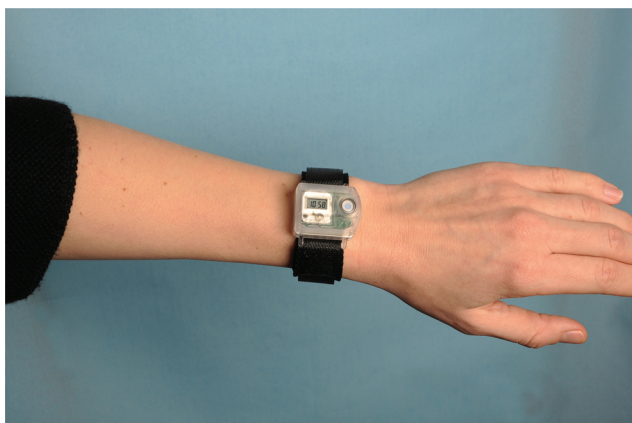
Fig. 5 An example of an electronic dosimeter called the "SunSaver" developed by the Department of Dermatology, Bispebjerg Hospital, Copenhagen. 8 An example of the data obtained from the SunSaver is shown in Fig. 6. The sensor can measure every 8 th second and store an average of the last 75 measurements every 10 minutes along with the time. The measurement range of the dosimeter is 0.1 SED per hour to 23 SED per hour and it is battery-driven. The dosimeter can run for 145 days without maintenance, and the data can be transferred to a computer.
