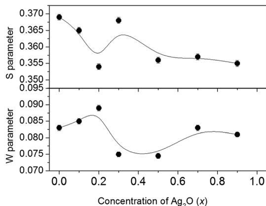
Fig. 14 The  $S$  and  $W$  parameters versus concentration ( $x$ ) of Ag<sub>2</sub>O in the samples.
