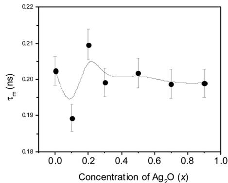
Fig. 11 The mean positron lifetimes versus concentration ( $x$ ) of Ag<sub>2</sub>O of the samples.
