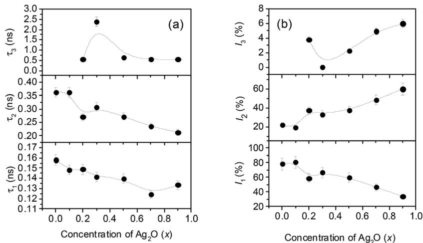
Fig. 9 (a) The positron lifetimes and (b) the relative intensities versus the concentration of Ag<sub>2</sub>O in the samples.
