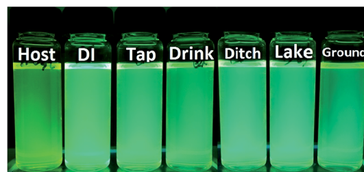
Fig. 6 The color changes observed by UV light of receptor L upon addition of 5 equiv. of \text{Hg}^{2+} in different source of water.
