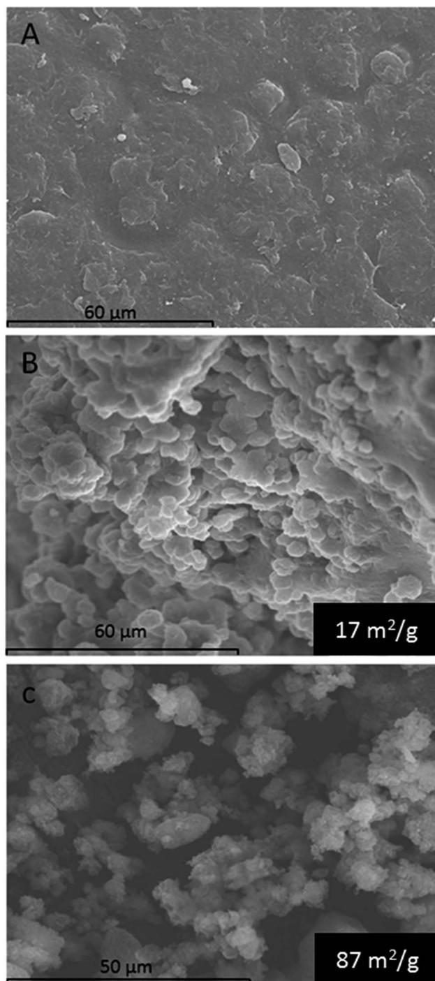
Fig. 3 SEM micrographs of a nylon pellet at 800 magnifications (A), material A at 800 magnifications (B) and material B at 1000 magnifications (C). Surface area ( $\text{m}^2 \text{g}^{-1}$ ) of B and C materials is also shown.
