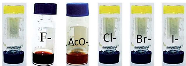
Fig. 8 Photograph of E6 organogels ( $8 \text{ mg mL}^{-1}$ ) upon adding of 10 equiv. of various anions in DMF, from left to right: none,  $\text{F}^-$ ,  $\text{AcO}^-$ ,  $\text{Cl}^-$ ,  $\text{Br}^-$ ,  $\text{I}^-$ .
