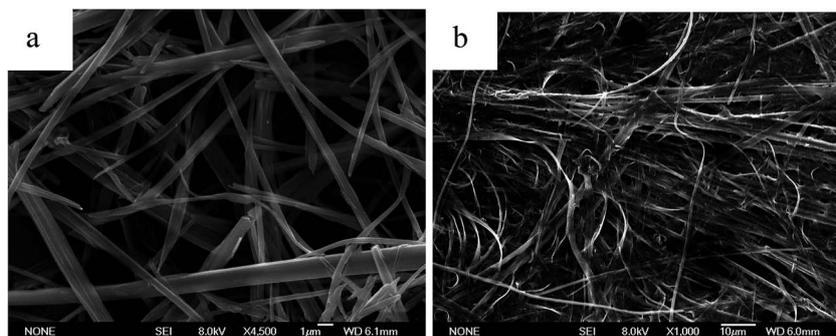
Fig. 1 SEM images of (a) **E6** xerogels (8 mg mL<sup>-1</sup>); (b) **E10** xerogels (11.5 mg mL<sup>-1</sup>) in DMF.
