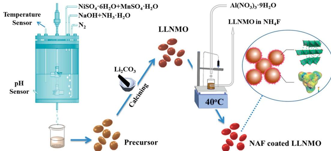
Scheme 1 Schematic diagram of the NAF-coated LLNMO synthesis process.
