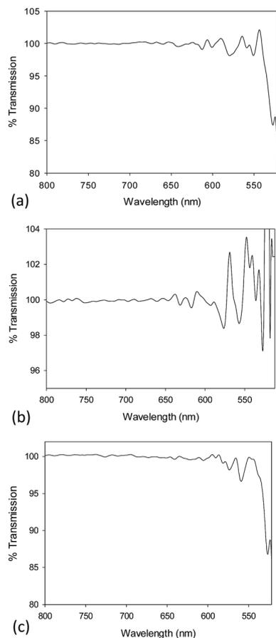
Fig. 2 (a) FT-IR spectrum for 10k PVP capped ceria NMs with Ce–O stretching was observed at c.  $550\text{ cm}^{-1}$ . (b) FT-IR spectra of 10k PVP capped zinc oxide NMs with Zn–O stretching peaks at just below  $600\text{ cm}^{-1}$  and that at  $517\text{ cm}^{-1}$ . (c) FT-IR spectra of 10k PVP capped copper oxide NMs with Cu–O stretching peaks at  $538\text{ cm}^{-1}$ ,  $557\text{ cm}^{-1}$  and  $570\text{ cm}^{-1}$ .
