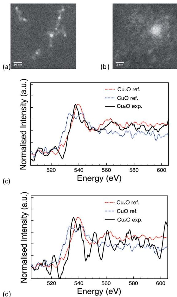
Fig. 5 (a) & (b) STEM image of PVP capped copper oxide NMs, (c) spectrum showing similarity to the O K-edge of  $\text{Cu}_2\text{O}$  & (d) spectrum showing no similarity to  $\text{Cu}_2\text{O}$  or  $\text{CuO}$  reference NMs.
