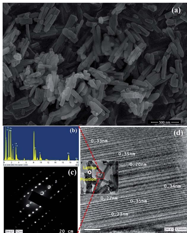
Fig. 3 (a) FESEM image, (b) EDS spectrum, (c) SAED pattern and (d) lattice HRTEM of  $\alpha$ - $\text{MoO}_{3(0.03)}\text{-WO}_{3(0.36)}/\text{CdS}_{(0.61)}$  ternary photocatalyst.
