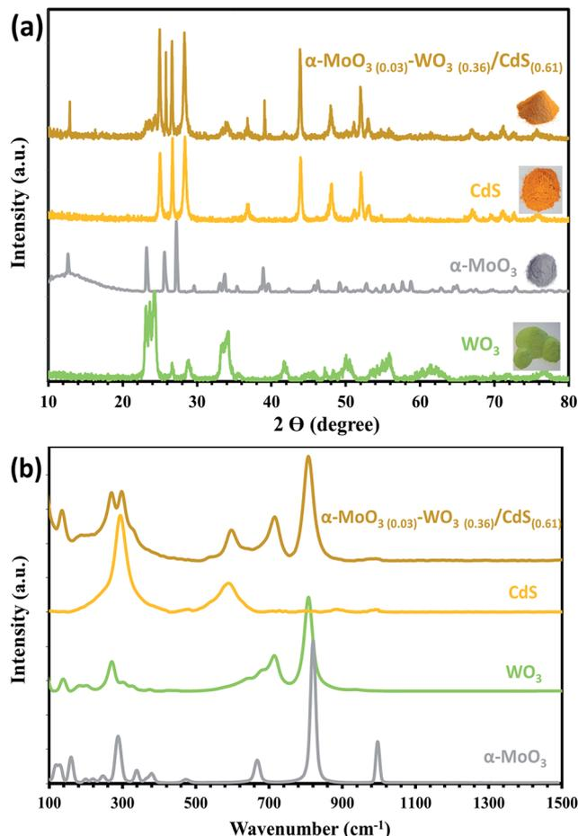
Fig. 2 (a) PXRD and (b) Raman patterns of  $\alpha$ - $\text{MoO}_3$ ,  $\text{WO}_3$ ,  $\text{CdS}$ , and the  $\alpha$ - $\text{MoO}_{3(0.03)}\text{-WO}_{3(0.36)}/\text{CdS}_{(0.61)}$  nanostructure photocatalysts.
