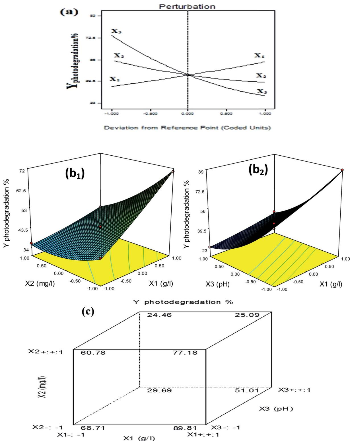
Fig. 5 Graphical diagrams of (a) the linear perturbation plots, (b) 3D surface contour plots, and (c) the cubic plots for benzoic photodegradation using  $\alpha$ -MoO<sub>3(0.03)</sub>-WO<sub>3(0.36)</sub>/CdS<sub>(0.61)</sub> as a function of visible light.
