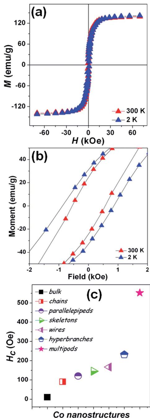
Fig. 5 Magnetic properties of stellated Co multipods. (a) The hysteresis loops of the Co multipods at 2 and 300 K. (b) The comparison of coercive fields at 2 and 300 K. (c) The comparison of the coercive fields for the different cobalt nanostructures with bulk.
