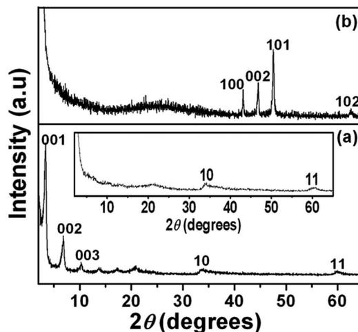
Fig. 1 XRD patterns of DS intercalated  $\alpha$ -cobalt hydroxide (a) and Co metal obtained on solvothermal reduction (24 h) of colloidal dispersion of DS intercalated  $\alpha$ -cobalt hydroxide (b). The *in situ* XRD pattern of the colloidal dispersion of DS intercalated  $\alpha$ -cobalt hydroxide in 1-butanol is shown as inset in (a).
