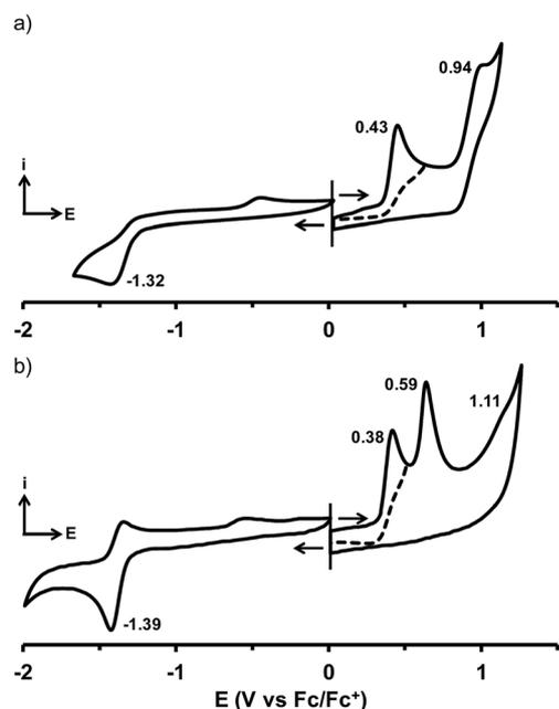
Fig. 2 Cyclic voltammograms of (a) 18 and (b) 31 in DCM containing 0.1 M of (*n*-Bu)<sub>4</sub>NPF<sub>6</sub> (scan rate of 100 mV s<sup>−1</sup>).
