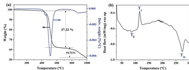
Fig. 5 TG-DSC analysis of the final l-PPS<sub>6</sub>/nano-HA<sub>4</sub> composite.
