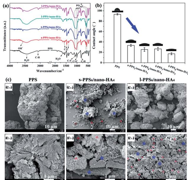
Fig. 3 FT-IR spectra (a) and water contact angle (b) of s-PPS/nano-HA and l-PPS/nano-HA binary composite. SEM images (c) of s-PPS<sub>6</sub>/nano-HA<sub>4</sub> and l-PPS<sub>6</sub>/nano-HA<sub>4</sub>.
