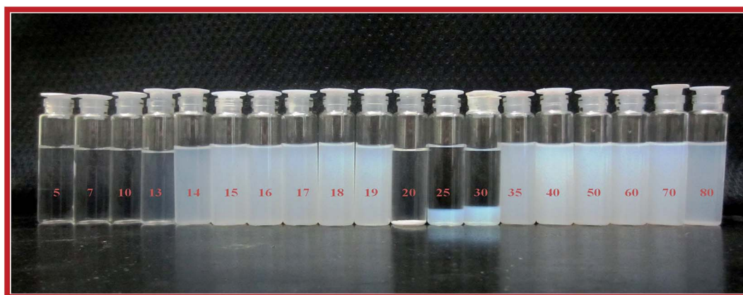
Fig. 2 Image of DS/ C_{16}VnImBr solutions at a constant final surfactant concentration (20 mmol) and variable [DS] from 5 to 80 mmol. The final [DS] are written in red numbers.
