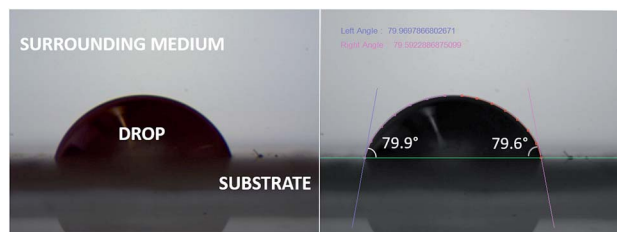
Fig. 3 Extraction of contact angle from obtained images of oil/water drop on the given substrate (micro-patterned or flat) kept underwater or in air using the tangent method.
