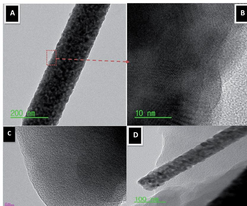
Fig. 4 Normal TEM (A) and HR TEM image for the red marked area (B). Panels (C) and (D) display normal TEM images of the pristine activated carbon and AC/Zr 10% nanocomposite, respectively.
