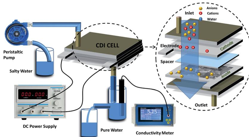
Fig. 1 Schematic of the capacitive deionization (CDI) setup.
