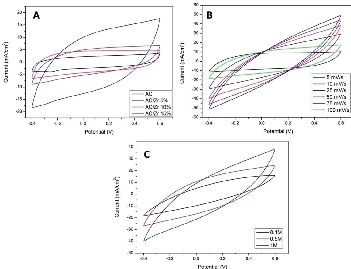
Fig. 7 (A) Cyclic voltammograms (CV) for the fabricated electrodes at a scan rate of  $10 \text{ mV s}^{-1}$  in a  $1 \text{ M NaCl}$  aqueous solution and (B) for the AC/Zr 10% electrode at various scan rates in a  $1 \text{ M NaCl}$  aqueous solution. (C) Comparative CV curves for the AC/Zr 10% electrode at various NaCl concentrations at a scan rate of  $50 \text{ mV s}^{-1}$ .
