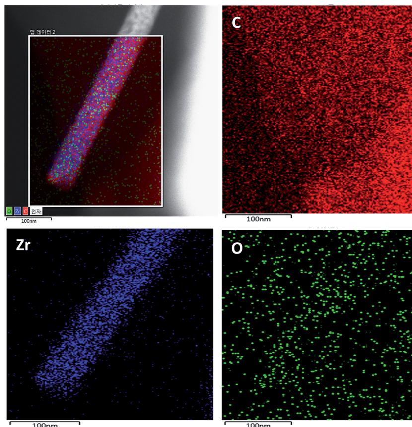
Fig. 5 TEM mapping of the AC/Zr 10% nanocomposite.
