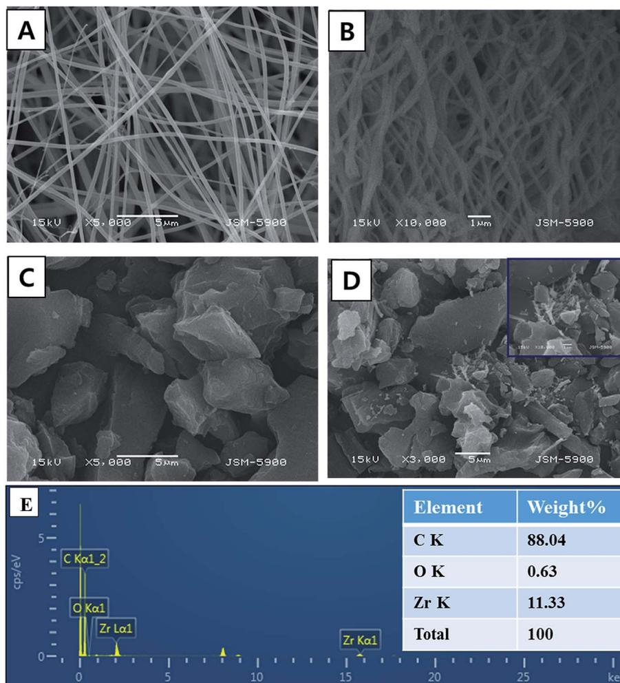
Fig. 2 (A and B) SEM images of: the Zr(Iso)/PVAc electrospun nanofiber mat and pure ZrO<sub>2</sub> nanofibers after calcination, (C) pristine activated carbon, and (D) AC/ZrO<sub>2</sub> 10% (inset is high magnification). (E) TEM EDX analysis for the AC/ZrO<sub>2</sub> 10%.
