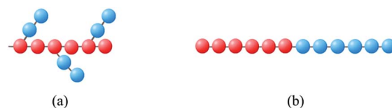
Fig. 1 Schematic representation of (a) comb-like block copolymer, (b) linear block copolymer. Hydrophobic backbone, red beads; hydrophilic side chains, blue beads.
