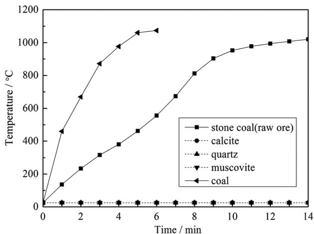
Fig. 4 Heating characteristics of the pure minerals.
