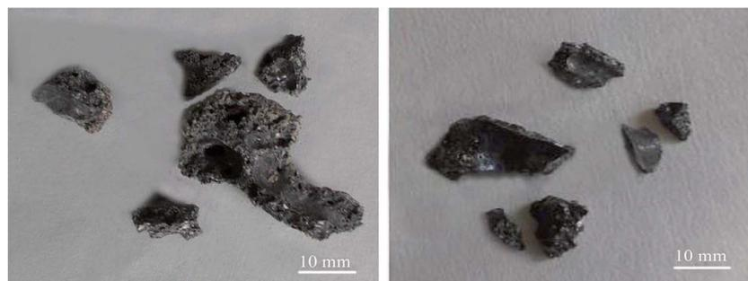
Fig. 8 Sintering phenomenon of stone coal during the microwave roasting process.
