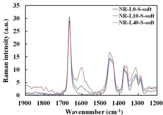
Fig. 1 Raman spectra of NR-L0-S-soft, NR-L10-S-soft and NR-L40-S-soft.
