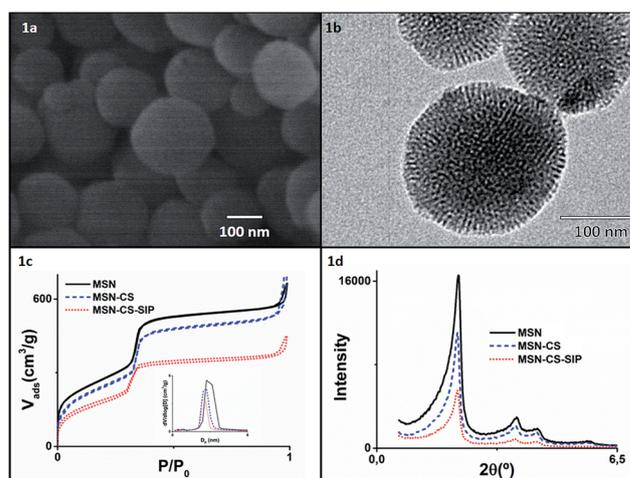
**Fig. 1** (a) SEM images of MSNs; (b) TEM images of MSNs; (c) nitrogen adsorption and desorption isotherms of MSN (black solid line), MSN-CS (blue dashed line) and MSN-CS-SIP (red dotted line) (inset: pore size distribution determined by the BJH method from the desorption branch of the isotherm); (d) XRD patterns of MSN (black solid line), MSN-CS (blue dashed line) and MSN-CS-SIP (red dotted line).
