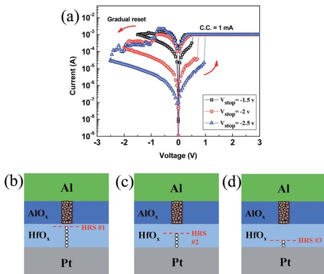
Fig. 5 (a) Typical  $I$ - $V$  curves of  $\text{AlO}_x/\text{HfO}_x$  bilayer structure measured at different reset stop voltages to show controllability of filament. (b-d) Schematic representation of resistive switching mechanism for 3 different HRS #1–3, respectively.
