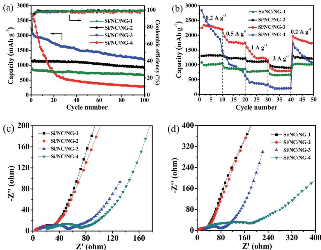
Fig. 5 Electrochemical performance of various Si/NC/NG electrodes measured in the voltage range of 0.01–1.5 V. (a) Cycling performance of at a current density of  $0.5 \text{ A g}^{-1}$ , (b) rate capability at different current densities, (c) Nyquist plots before cycling, (d) Nyquist plots after rate capability tests.
