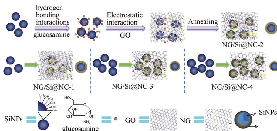
Fig. 1 The preparation procedure for Si/NC/NG nanohybrids.
