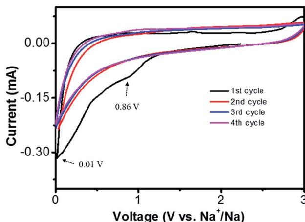
Fig. 4 Cyclic voltammograms of the Na/NCF half cells at 0.5 mV s<sup>-1</sup> scan rate, voltage 0.001–3 V.
