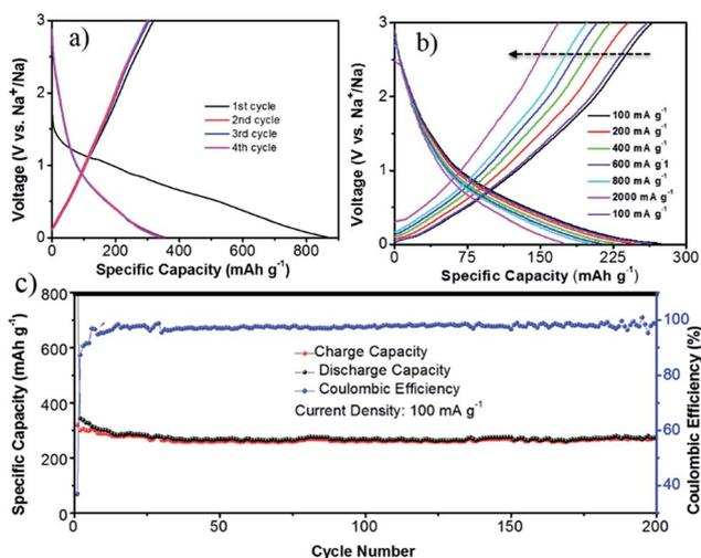
Fig. 5 Sodium storage performance of the NCF: discharge-charge profiles for the first 4 cycles at a current density of  $100 \text{ mA g}^{-1}$  (a); rate capability at various current densities ( $100$ – $2000 \text{ mA g}^{-1}$ ) (b); and cycling performance (c).
