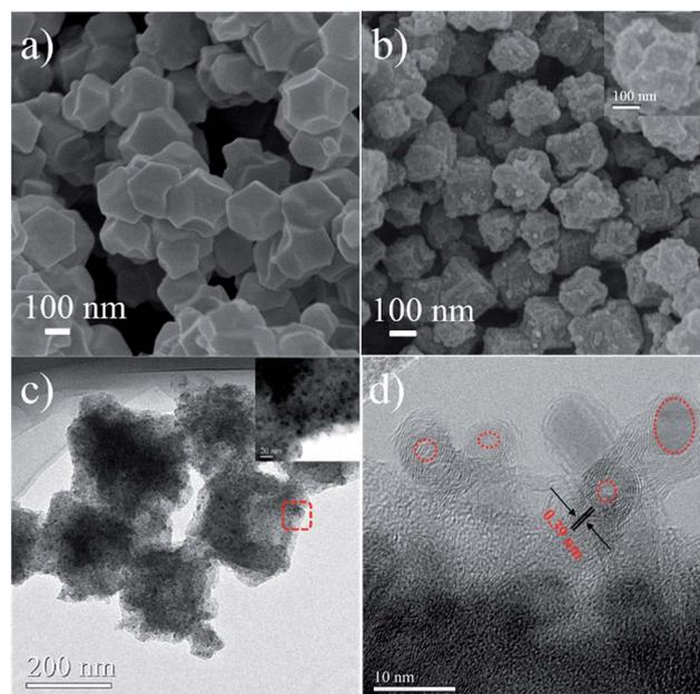
**Fig. 1** SEM images of the ZIF-67 precursor (a), and the as-obtained 3D NCF (b), with the inset showing the hollow structure of the polyhedra. TEM (c) and HR-TEM (d) images of the NCF. The inset to (c) is an enlargement of the indicated area, and the red circles in (d) mark the hollow centers of the nanospheres.
