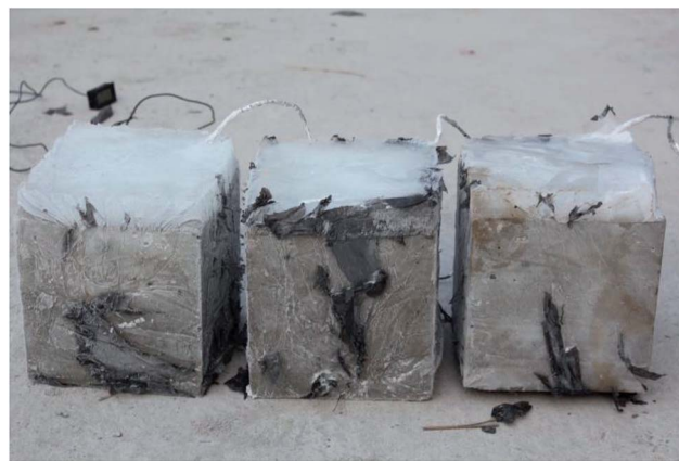
Fig. 7 Specimens covered with ice layer.
