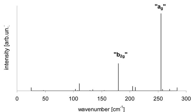
Fig. 10 Calculated vibronic intensities in the spectrum of Tr molecule in a 2,3-DCN crystal estimated as the square of the scalar products of the vectors describing geometrical differences in the electronic ground  $S_0$  and lowest excited  $S_1$  states (see Table S9†).
