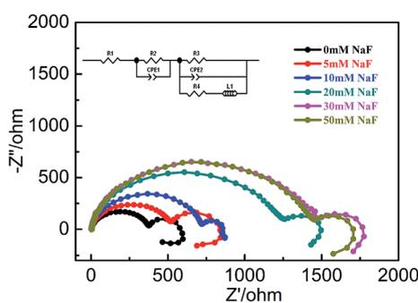
**Fig. 3** EIS plots of AZ31B Mg alloy in composite electrolyte solution (MgSO<sub>4</sub> : Mg(NO<sub>3</sub>)<sub>2</sub> = 7 : 93) with different concentrations of NaF.
