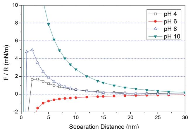
Fig. 9 The normalized forces between the surfaces of 6H-SiC and ceria particles as a function of separation distance at different pH values. The surface potentials of the SiC plate and ceria particles are 30 and 43 mV at pH 4,  $-56$  and 24 mV at pH 6,  $-96$  and  $-2$  mV at pH 8,  $-125$  and  $-40$  mV at pH 10, respectively. The Hamaker constant is  $8.5 \times 10^{-20}$  J and the background electrolyte is 1 mM  $\text{KNO}_3$ .
