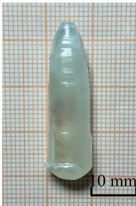
Fig. 1 Photograph of KNN47 single crystal grown via TSSG.
