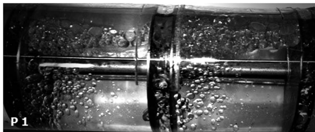
Fig. 2 Picture of drop size in the horizontal pulsed sieve plate column (c → d).
