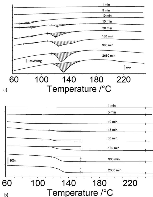
Fig. 1 (a) DSC measurements of heat flow for 17  $\mu\text{m}$   $I_2O_5$  at different exposure time intervals to 80% RH as indicated on the curves; and, (b) TG measurements of mass change for 17  $\mu\text{m}$   $I_2O_5$  at different exposure time intervals to 80% RH as indicated on the curves. Onset and end temperature for measurements of mass loss are determined by endotherm onset and end temperatures.
