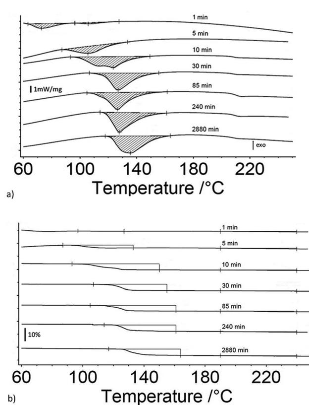
Fig. 2 (a) DSC measurements of heat flow for 5  $\mu\text{m}$   $I_2O_5$  at different exposure time intervals to 80% RH as indicated on the curves; and, (b) TG measurements of mass change for 5  $\mu\text{m}$   $I_2O_5$  after different exposure time intervals to 80% RH as indicated on the curves. Onset and end temperature for measurements of mass loss are determined by endotherm onset and end temperatures.
