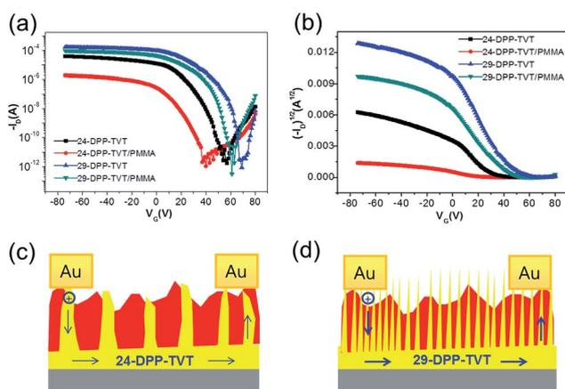
Fig. 4 (a)  $-I_D$ , (b)  $(-I_D)^{1/2}$  versus  $V_G$  characteristics for the FETs based on 24-DPP-TVT film, 24-DPP-TVT/PMMA blend film, 29-DPP-TVT film, and 29-DPP-TVT/PMMA blend film.  $V_D$  is fixed at  $-80\text{ V}$ . Schematic drawings of charge injection and transport in the 24-DPP-TVT/PMMA blend film (c), and 29-DPP-TVT/PMMA blend film (d).
