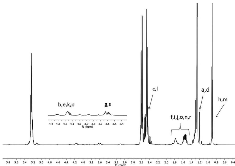
Fig. 2  $^1\text{H}$  NMR spectrum of oligo(3-hydroxybutyrate-co-3-hydroxyhexanoate) diols obtained *via* reduction of high molar mass PHBHx biopolyester. Refer to Scheme 2 for the chemical structures of the oligomers.
