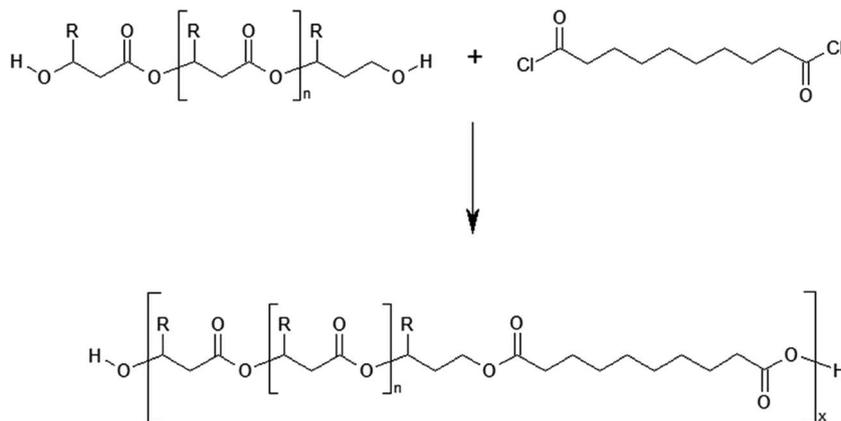
Scheme 4 Polycondensation reaction of PHBHx oligodiols with sebacoyl chloride. R = CH<sub>3</sub> for 3HB units or R = C<sub>3</sub>H<sub>7</sub> for 3HH units.
