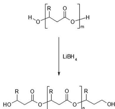
Scheme 1 Reduction reaction of poly(3-hydroxybutyrate-co-3-hydroxyhexanoate) by lithium borohydride (R = CH<sub>3</sub> for 3HB units or R = C<sub>3</sub>H<sub>7</sub> for 3HH units).
