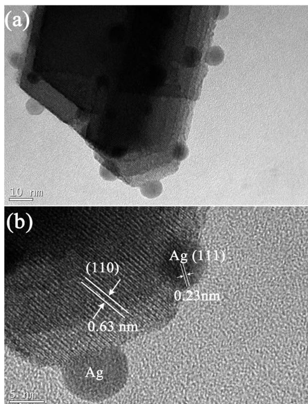
Fig. 3 (a) A typical TEM image of a rod-like building block of the urchin-like Ag/WO<sub>3</sub>·0.33H<sub>2</sub>O, (b) the corresponding HRTEM image.
