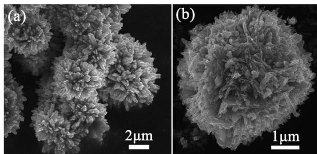
Fig. 2 SEM images of the as-synthesized Ag/WO<sub>3</sub>·0.33H<sub>2</sub>O. (a) Low-magnification, (b) high-magnification.
