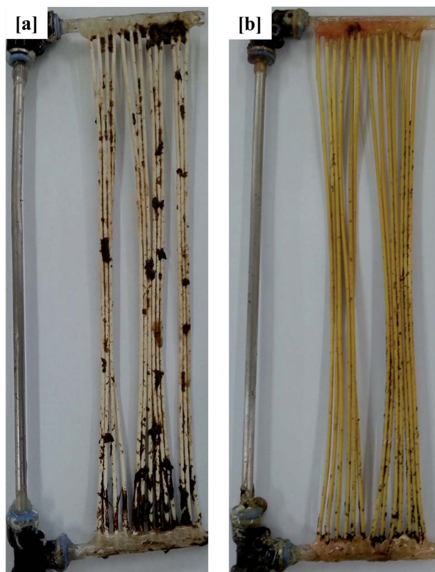
Fig. 3 Photographs of the membrane module from the (a) control MBR (w/o curcumin) and (b) test MBR (with curcumin). The membrane modules were removed when the TMP of the control MBR reached 40 kPa.
