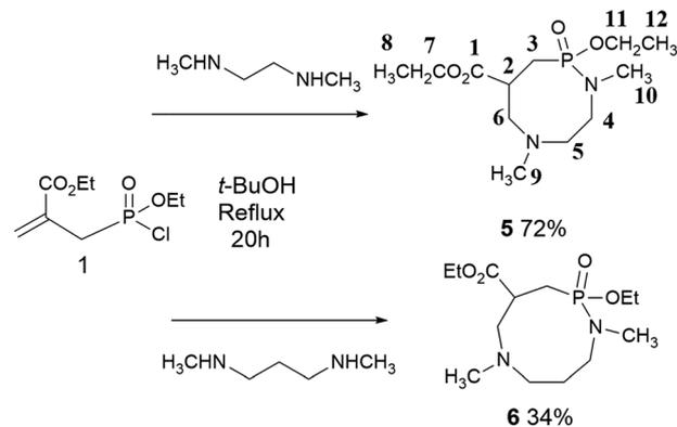
Scheme 1 First synthesis of diazaphosphocane **5** and diazaphosphonane **6**.
