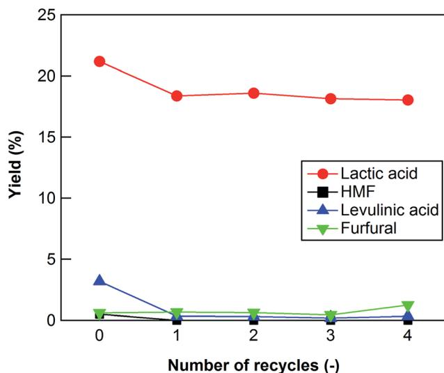
**Fig. 4** Cellulose conversion using a recycled ZrO<sub>2</sub> catalyst. Reaction conditions: 0.5 g ball-milled cellulose, 1 g ZrO<sub>2</sub> (ZRO-7), 50 g water, 473 K reaction temperature, 6 h reaction time.
