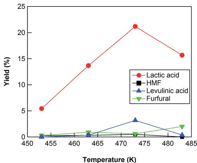
Fig. 2 Cellulose conversion using a  $\text{ZrO}_2$  catalyst as a function of reaction temperature. Reaction conditions: 0.5 g ball-milled cellulose, 1 g  $\text{ZrO}_2$  (ZRO-7), 50 g water, 6 h reaction time.
