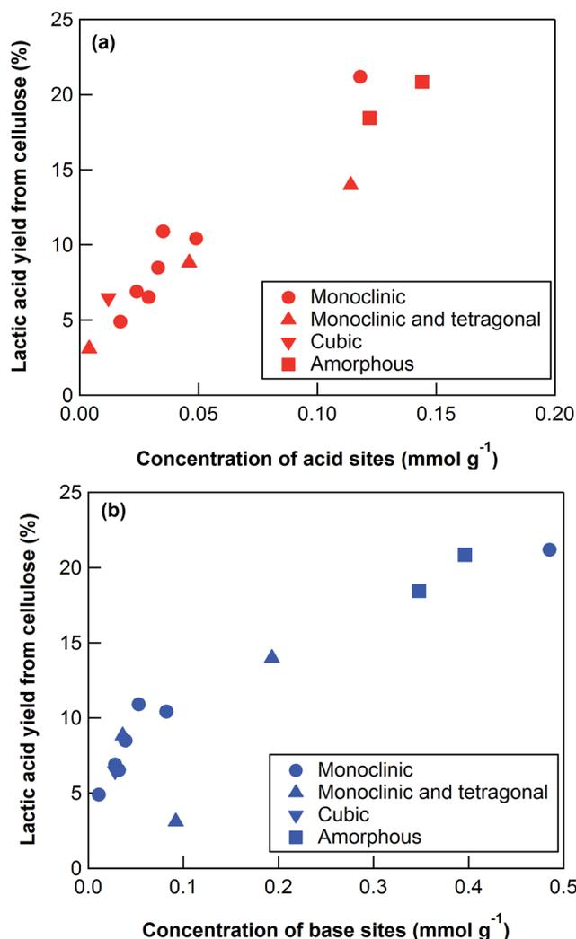
Fig. 3 Lactic acid yield from cellulose using  $\text{ZrO}_2$  catalysts as a function of the concentration of (a) acid and (b) base sites. Reaction conditions: 0.5 g ball-milled cellulose, 1 g  $\text{ZrO}_2$ , 50 g water, 473 K reaction temperature, 6 h reaction time.
